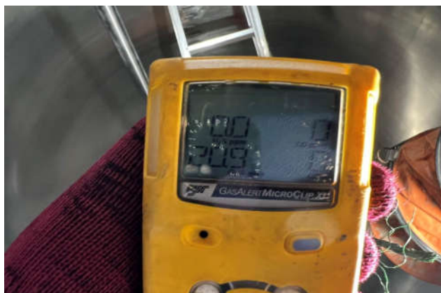
Measure the oxygen level inside the tank (Oxygen (O2), (19.5-23.5%)) 槽内酸素濃度
