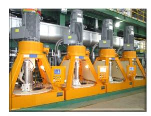
Fully automatic batch type centrifuges
